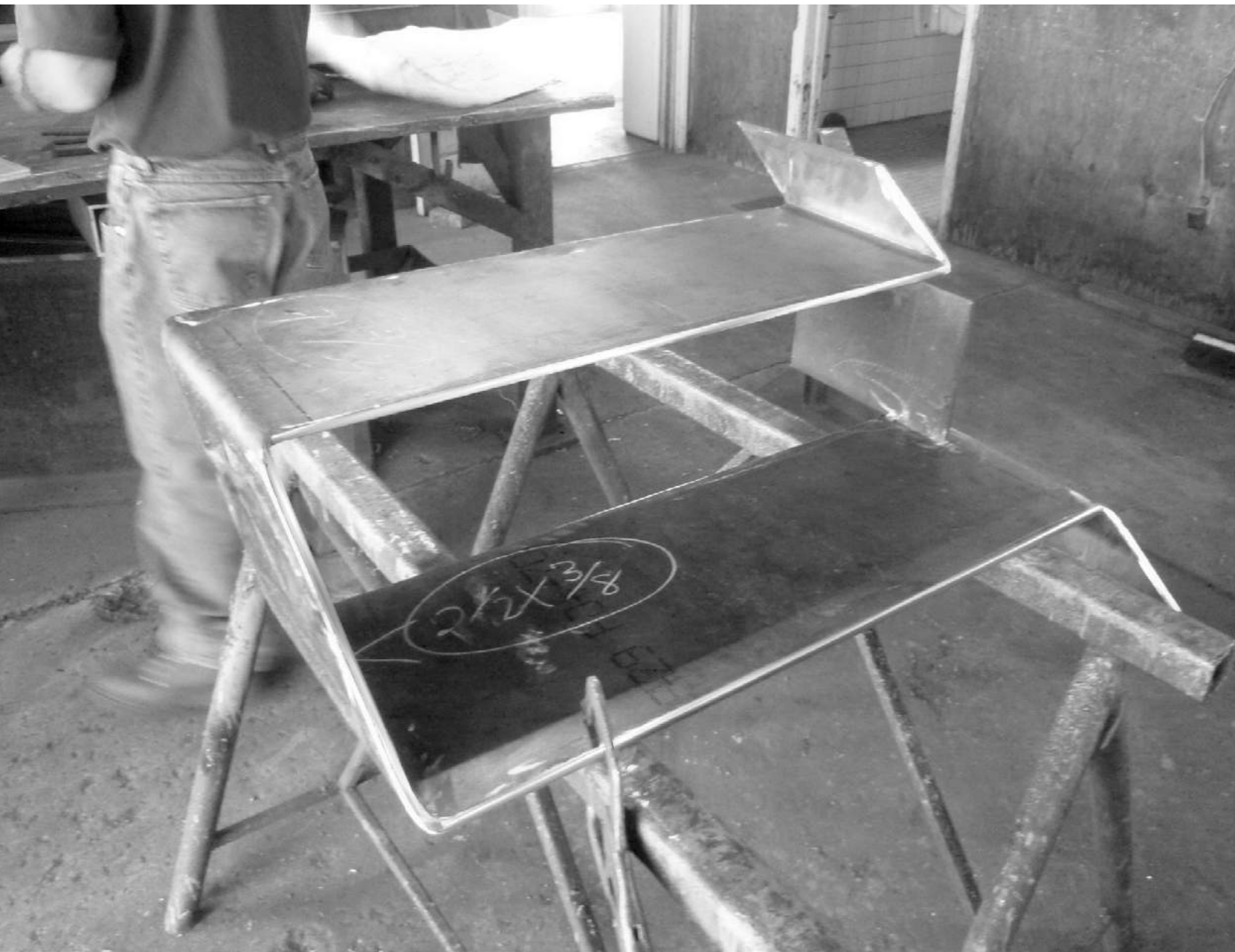
one of six units diagonally sliced from one large pre-folded steel sheet
